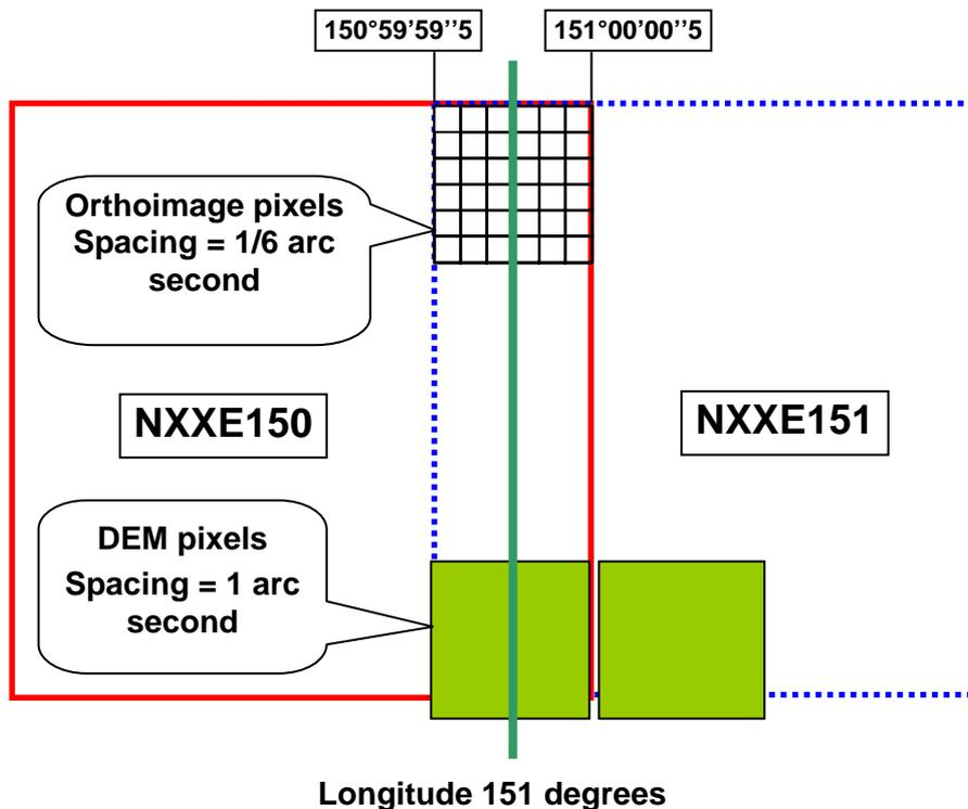
**Important :** Orthoimage data overlapping the neighbouring tiles (three rows/columns along the four edges of the tile) are only given to ensure that the DEM and orthoimage register exactly. They are provided for information purposes only and Spot Image does not warrant their fitness for any particular use.
